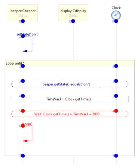
A collection of locations from different lifelines that are subjected to the requirement that none of these lifelines can proceed past its location in the synchronization point until all other instances reach their locations in the synchronization point.
